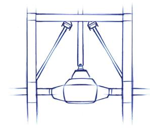
**Truck Trailing Arm** – While similar to the 2-link, the angled lower bars separates this design from the limited 2-link. This system is capable of articulation, which makes it much more viable for street use. It was used on the early GM pickups and is still used as the only rear suspension accepted in NASCAR. This design, like the 2-link, leaves lots of room for the fuel tank, exhaust, and even a back seat.
