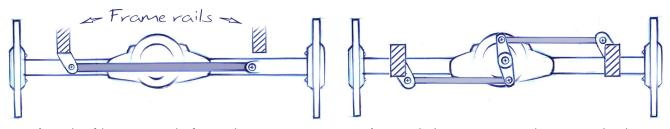
A panhard bar is a simple device that mounts to the frame on one side and the axle on the opposite side.
