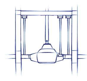
**Parallel 3-link** – Commonly used on 60's GM cars, this design can help in situations where space is tight. The single upper bar can be installed on either side of the axle to make room for the fuel tank or whatever else might be in the way. The downfall of the design is that it is not ideal for high horsepower installations.
