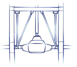
The Parallel 3-link, Parallel 4-link, Wishbone 3-link, and the triangulated 4-link can all potentially look the same from a side view.
